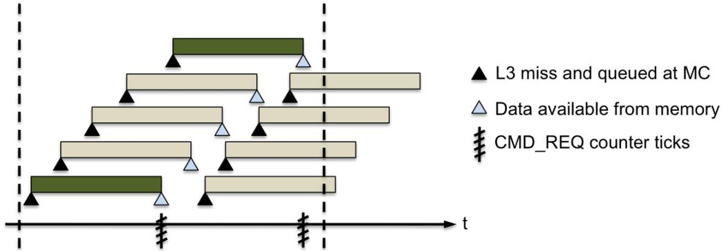
Figure 2: Example: Tracking of memory requests using counters
