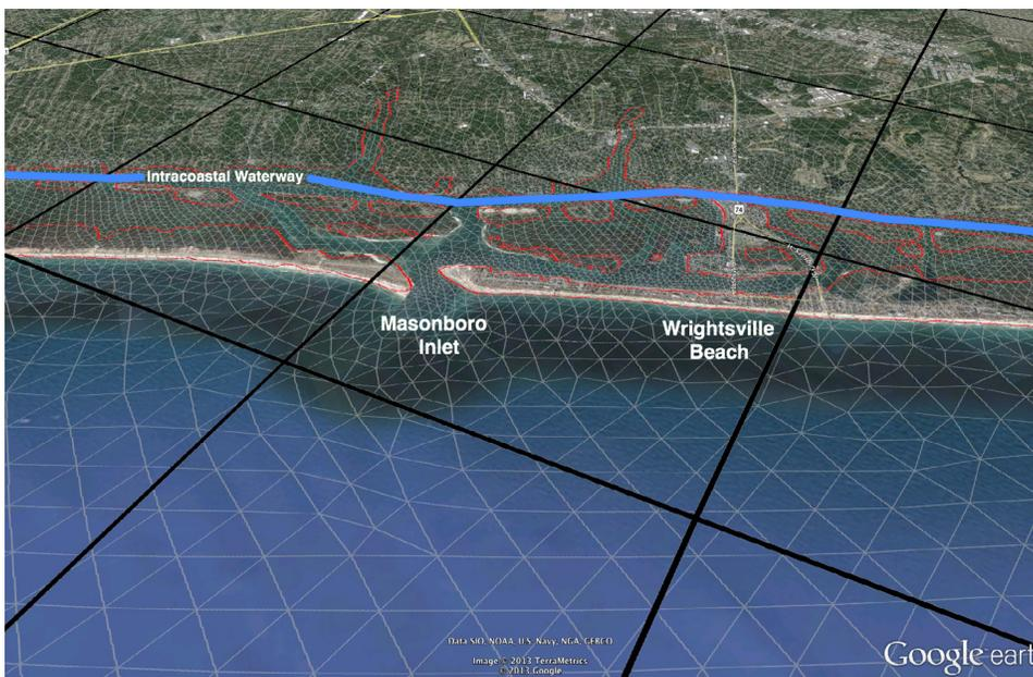
**Figure 1:** ADCIRC (gray triangles) and SLOSH (black squares) model grids in the Wrightsville Beach, NC area. Because ADCIRC uses triangles as its descriptive basis, it allows flood prediction at a much greater level of detail than the coarser SLOSH model, which uses squares. The red line is the coastline in ADCIRC's grid.
