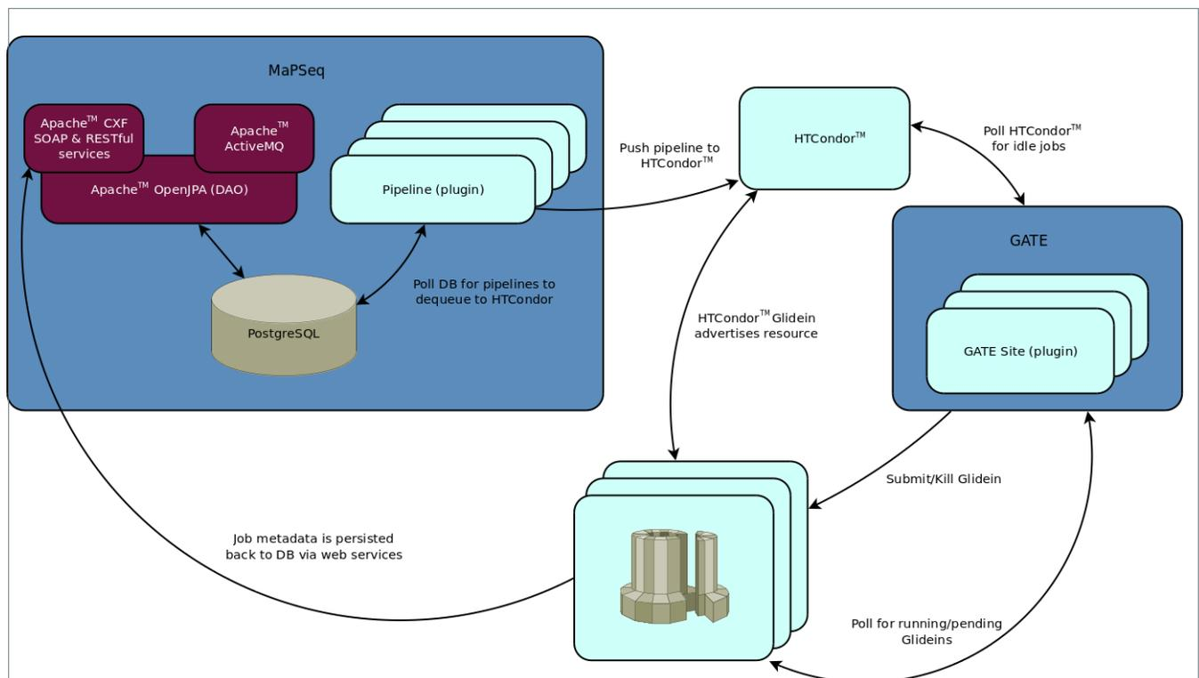
**Figure 1.** A schematic showing the architecture of MaPSeq, with arrows depicting the flow of information. DB = database; GATE = Gate Access Triage Engine; RESTful = Representational State Transfer; SOAP = Simple Object Access Protocol.
